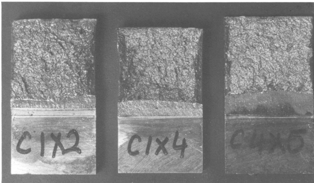
Figure 13 Fracture surfaces for 25 mm thick specimens of steel C.
