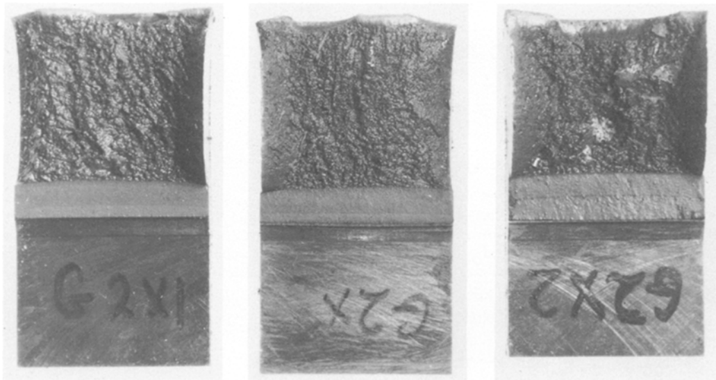
Figure 16 Fracture surfaces of 25 mm thick specimens of steel G.
